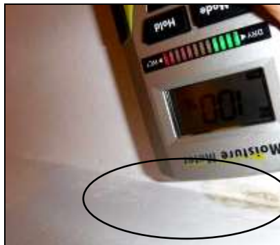
Figure 4 Mold like spots and active leak/moisture (100%). Recommend a licensed plumber evaluate all sources and advise on repairs. Recommend contacting the Association to see if unit above is the source or in this unit.
